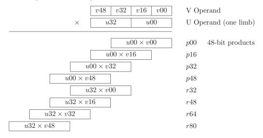
p32 and r32 can be summed using floating-point addition, and likewise p48 and r48. p00 and p16 can be summed with r64 and r80 from the previous iteration.
