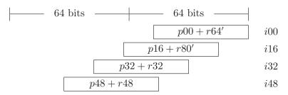
The challenge then is to sum these efficiently and add in a carry limb, generating a low 64-bit result limb and a high 33-bit carry limb (i48 extends 33 bits into the high half).
