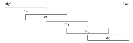
The  $w_i$  coefficients could be formed by a simple set of cross products, like  $w_4 = x_2y_2$ ,  $w_3 = x_2y_1 + x_1y_2$ ,  $w_2 = x_2y_0 + x_1y_1 + x_0y_2$  etc, but this would need all nine  $x_iy_j$  for i, j = 0, 1, 2, and would be equivalent merely to a basecase multiply. Instead the following approach is used.
