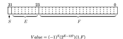
Figure B.1: IEEE single-precision floating-point format
