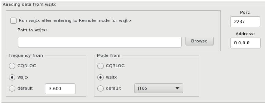
Cqrlog acts as UDP server that listens at specified address. It defaults to 127.0.0.1 (localhost) but can be changed to any network interface address the PC running cqrlog has.
