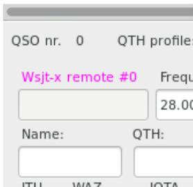
When remote mode is selected it shows last received WSJT-X packet type number after text “Wsjt-x remote” text. Also color of text changes while receiving packets. These will show you that UDP link is alive between these programs.
