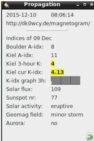
This propagation form is an alternative showing details from dk0wcy page with 3 hour graphical display of K-index.
