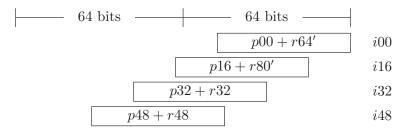
The challenge then is to sum these efficiently and add in a carry limb, generating a low 64-bit result limb and a high 33-bit carry limb (i48 extends 33 bits into the high half).
