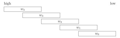
The  $w_i$  coefficients could be formed by a simple set of cross products, like  $w_4 = x_2y_2$ ,  $w_3 = x_2y_1 + x_1y_2$ ,  $w_2 = x_2y_0 + x_1y_1 + x_0y_2$  etc, but this would need all nine  $x_iy_j$  for i, j = 0, 1, 2, and would be equivalent merely to a basecase multiply. Instead the following approach is used.
