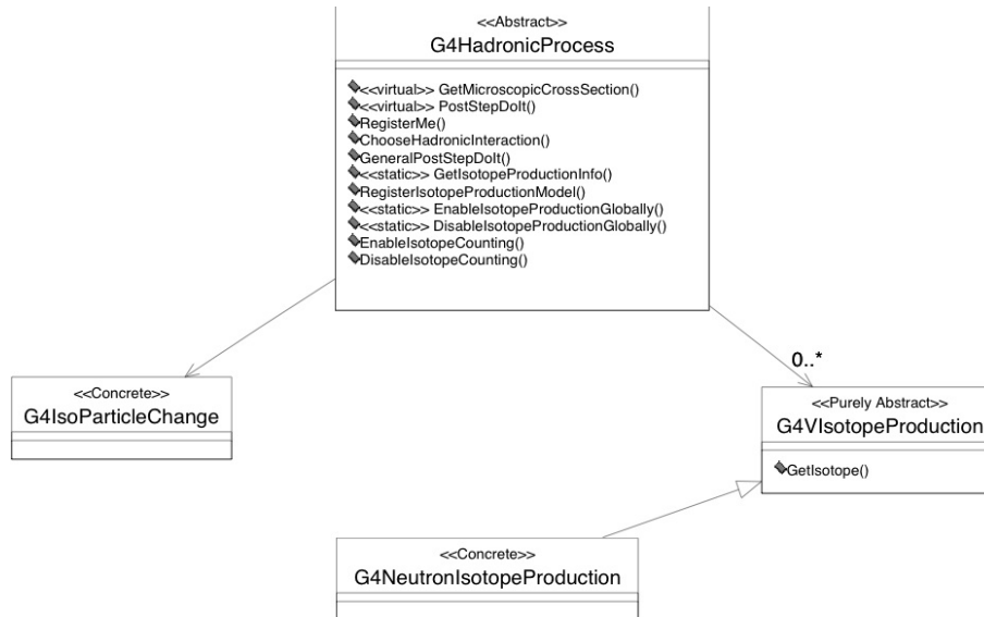
Fig. 3.6: Level 2 implementation framework of the hadronic category of GEANT4; isotope production aspect
