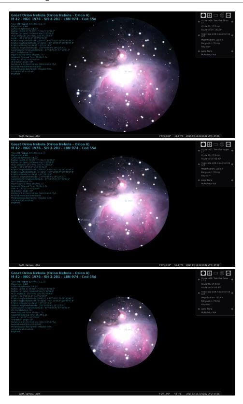
Figure 15.17: Comparing apparent fields of view of (top) a 17 mm Tele Vue Ethos eyepiece with an aFOV of  $100^{\circ}$ . Magnification is  $119.5 \times$ . (center) a 17 mm Tele Vue Nagler eyepiece with an aFOV of  $82^{\circ}$ . Magnification is  $119.5 \times$ . (bottom) a 17.3 mm Tele Vue Delos eyepiece with an aFOV of  $62^{\circ}$ . Magnification is  $117.5 \times$ .
